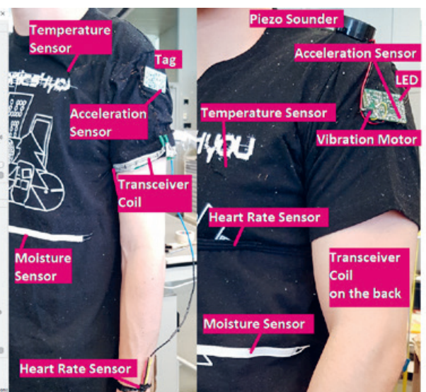
Demonstration setup with software on the left and textile-based hardware used for worker protection on the right. Own presentation
