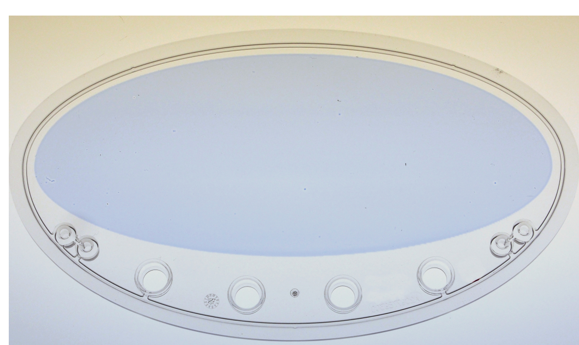
Anti-scratch coating colored for homogeneity tests.
