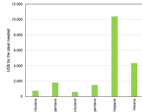
Price of steel needed after machining for a compressor at  $T_c=120^\circ\text{C}$  and a cooling capacity of 500 kW
