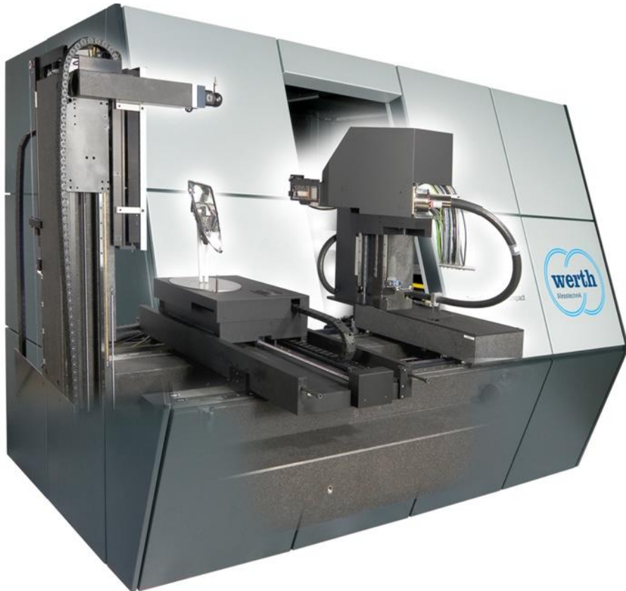
Werth TomoScope® L L = 419 mm; Ø = 212 mm
