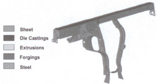
Figure 21: Aluminium cockpit carrier for high volume production with a transverse beam joined by non-vacuum electron beam welding
