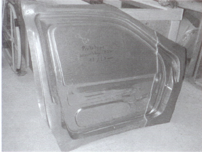
Figure 9: Friction Stir Welding, 5182 alloy, tailored blanks (1,2 mm/2,5 mm)
