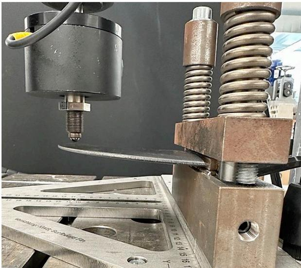
Figure 5. Set-up for local stiffness measurement
