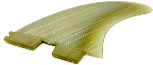
Figure 2. Surf fin used as practical geometry (rPET)
