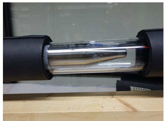
Figure 2.13: Left: Laboratory setup to test the coated tubes under flow conditions; right: tip of sample tube
