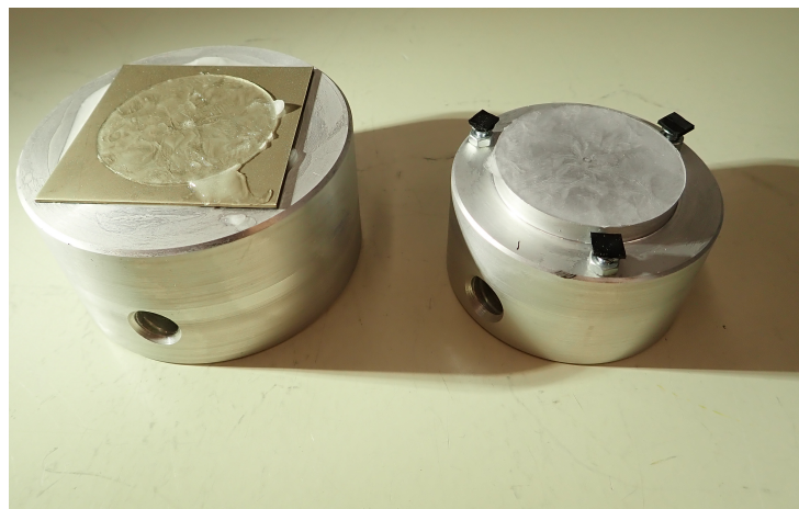
Figure 3.6: Ice adhesion test with force perpendicular to the sample surface: cohesive ruptures in the ice lead showing remaining ice on both sides: coating (left) and upper sample holder (right).
