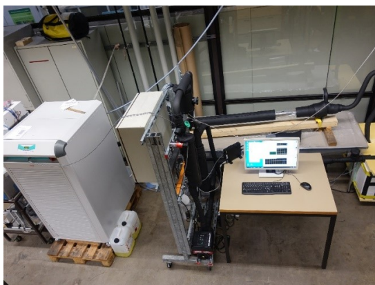
Figure 2.13: Left: Laboratory setup to test the coated tubes under flow conditions; right: tip of sample tube
