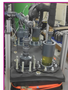
Gasketed heat exchanger (supercooler) used to supercool water.
