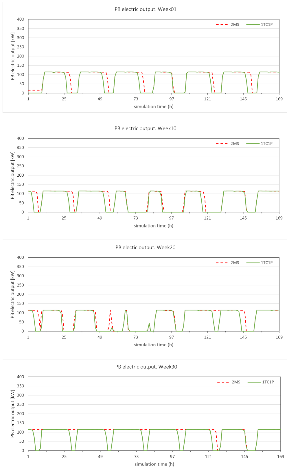
Figure 25: Electricity produced by the power block for the thermocline CSP plant (1TC1P), in continuous green line, compared with the two-molten salts CSP plant (2MS), in dashed red line, for different weeks.
