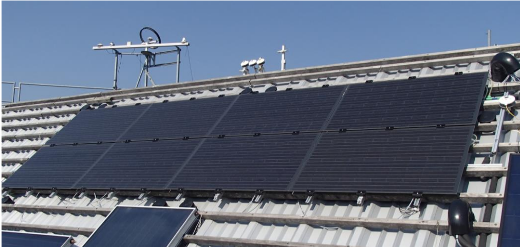
Figure 45: Trial system at the SPF Institute for Solar Technology. 2 PV modules installed at the left-hand edge of the field plus 6 PVT modules with the same electrical specifications.
