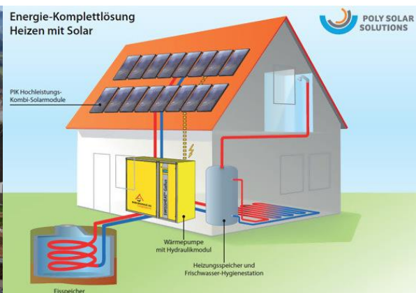
Figure 54: View of one of the apartment houses in the “Freihof” complex in Andwil, with diagram of heat supply system. Photo: Bion Bauhaus AG, Illustration: Poly Solar Solutions AG.
