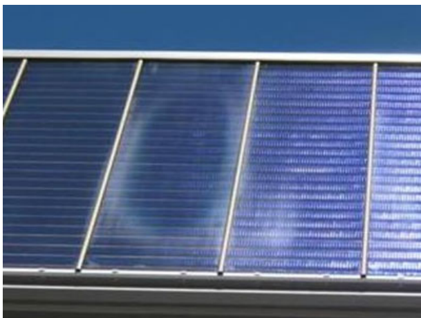
Fig. 1 Different forms of outgassing as they can be caused by thermal insulation.
