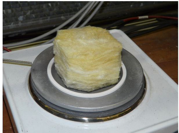
Fig. 4: Test sample on the hot aluminium plate. The black fleece is in direct contact with the plate.
