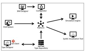
The proposed system's architecture. We focused on the configurator and data structures used between the tools.
