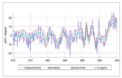
Orientation (only pitch) of the helicopter tracked by the extended Kalman filter. The estimated trajectory (green) is quite good compared to the raw measurement (blue).
