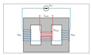
Variable inductance schematic with the different windings on an E-core
