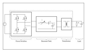
Schematic representation of a resonant circuit module Eigene Darstellung
