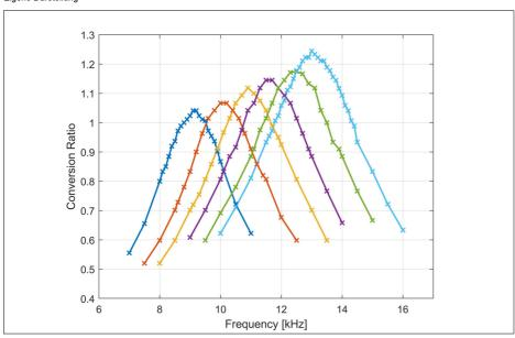
Modular conversion ratio measurement of three hardware modules connected in series Eigene Darstellung
