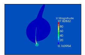
Velocity distribution around the blad at a TSR of 6
