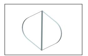
3D blade and tower geometry of the 17 m Darrieus VAWT
