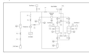
Recommended parallel setup of the new adsorption setup based on the research collected and trials ran Own presentment
