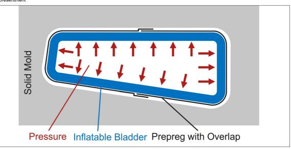
Schematic illustration of inflatable bladder process. Own presentment
