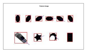
A binary image showing different clearly separated blobs. The image is overlaid with extracted feature data.
