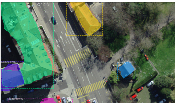
Bounding boxes and prediction masks generated by our Neural Network Own presentation
