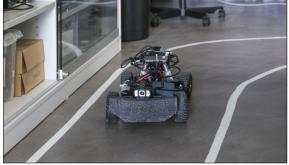
The built car driving autonomously within a lane using a neural network.
