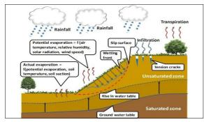
Figure 1: Mechanism of rainfall-induced slope failure
