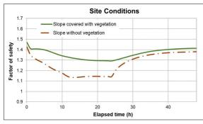
Figure 3: Factor of safety - Elapsed time, rainfall 22 mm/h for 24 h
