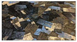
Material covered with release film after the double diaphragm forming process Own presentment
