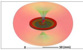
Simulated 3D antenna radiation pattern of the second prototype. Own presentmer
