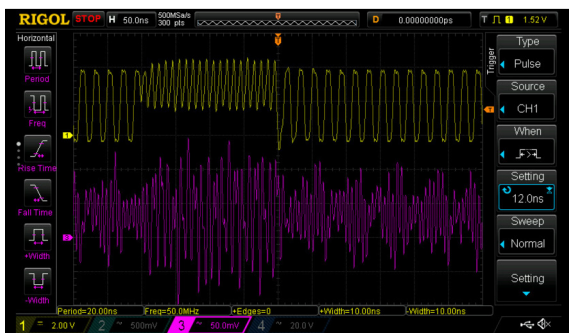
Clock Glitching Oscilloscope Screenshot Top: Clock signal with glitches, Bottom: CPU power consumption Own presentation
