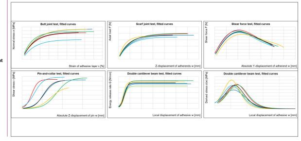
Reproducible experimental results representing the mechanical behaviour of the different bonded specimens Own presentment
