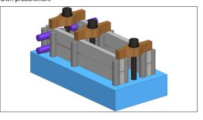
Multifunctional bonding and testing device for butt joint, scarf joint, shear and pin-and-collar tests. Own presentment
