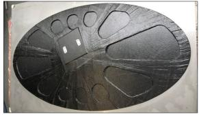
Manufactured disc as sandwich structure with integrated aluminum core for assembly Own presentment
