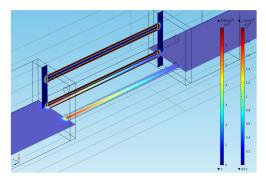
Frequency Displayed: 17.5 kHz Vertical Slice: Power Dissipation Losses Horizontal (W/m3); Slice: Power Intensity (W/m2)
