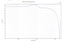
Loss in sound pressure level in dB between inlet and outlet of the perforation within the frequency band from 20 Hz to 20000 Hz
