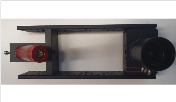
The developed laser triangulation sensor Own presentment
