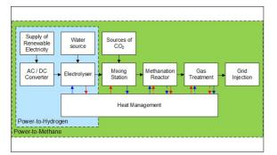
System boundary, Concept of a Power-to-Methane plant
