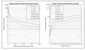
Geometric reactor volume as function of GHSV and cycle time.
