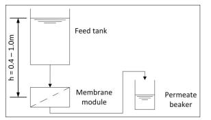
Fig. 1: Schematic of a GDM filtration process Own presentment
