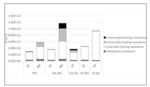
Fig. 3: Resistance caused by the membrane and different types of foulant at the end of the experimental period Own presentment
