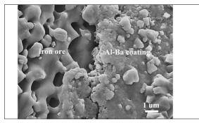
Figure 3: Scanning electron microscopy image of iron ore coated with aluminium-barium after one cycle. Own presentment
