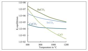
Figure 1: Constant equilibrium for the reaction of barium, strontium and calcium carbonate with HCl over temperature Own presentment
