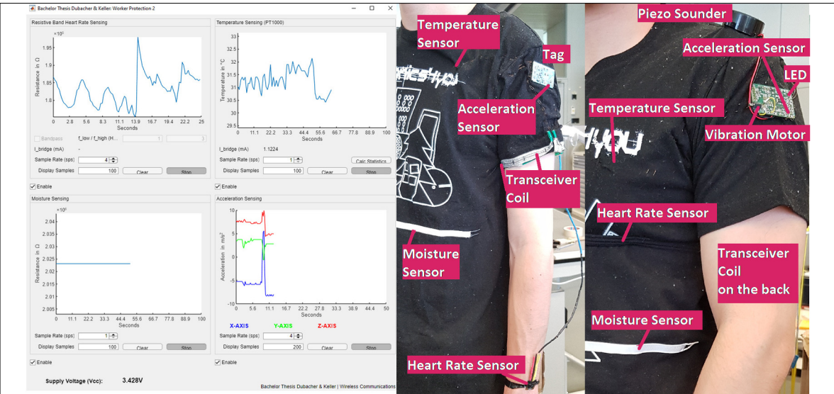
Demonstration setup with software on the left and textile-based hardware on the right used for worker protection. Own presentment
