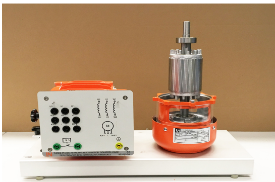
Actual stator and squirrel-cage rotor
