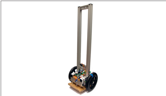
Completed Segway platform with the pendulum
