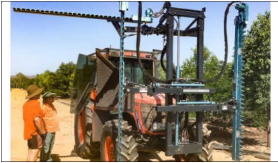
Current offered Ledgard Pruning medium-duty crank-drive cutter bar on a tractor Ledgard Pruning Systems
