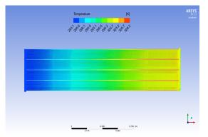
Water temperature contour normal to PVT plane of collector B
