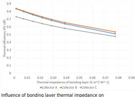
thermal collector efficiency
