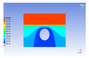
Cross section temperature contour of collector C
