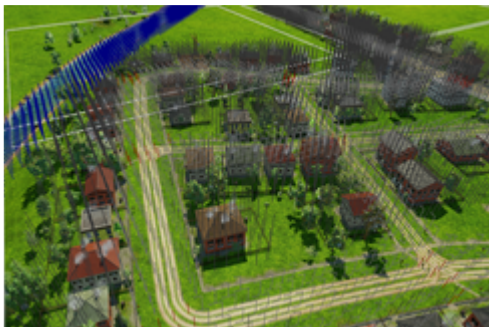
The visualization of the collision detection system. The vertical lines are color-code obstacles. Any obstacle could be dealt with appropriately.
