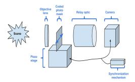
Design of the experimental setup showing the major components. The movement of the stage and the camera are synchronized.
