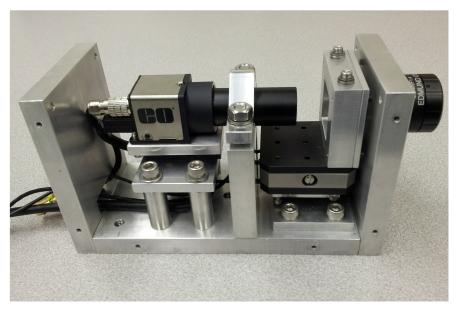
Fully assembled video camera prototype
