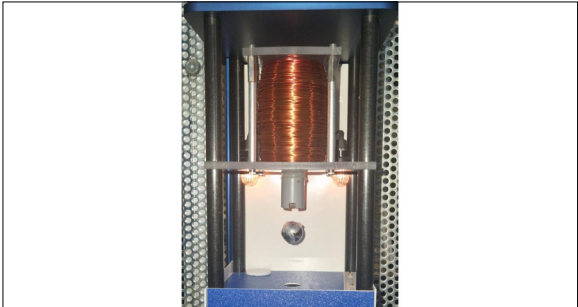
Figure 2: Picture of the magnetic levitation process balancing a magnetic ball using MPC. Own presentation
