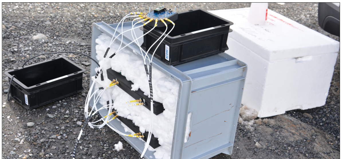
Figure 3: Field measurement setup showing the stripline sensors placed in the snowpack. Own presentation
