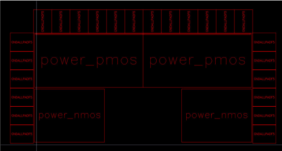
Layout of the high power transistors Own presentation
