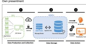
Fig. 1: Schematic of an energy plant monitoring data pipeline with a remote time series database. Own presentment
