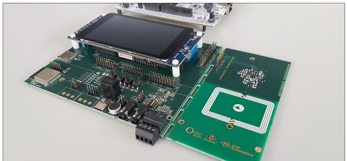
Fig. 3: Platform setup: green baseboard for all custom extensions, dev board on top: STM32F469I-Disco (or Nucleo-H755). Own presentation
