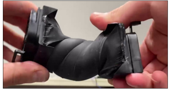
New Adhesive: No Failure at 540° Twist Own presentation
