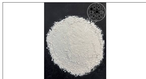
Catalyst Y used for the synthesis of methanol into hydrocarbons Own presentation
