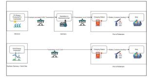
schematic visualization of the well-to-tank transport network scenario
