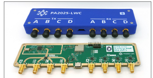
Figure 2: Realized dual LWC sensor with two back-to-back microstrip lines and two TX/RX port pairs. Own presentation
