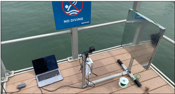
Experimental setup for the feasibility study with a stationary steel plate and opposing single-beam sonar sensor. Own presentation
