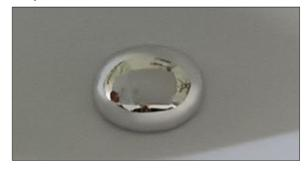
Image of liquid metal after reaction with carbon dioxide in bubble column reactor to form gallium oxide and solid carbon Own presentment
