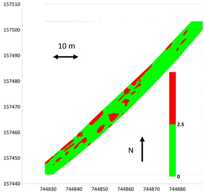
**Figure 3: Quotients of amplitudes top of concrete/top layer of rebar**
