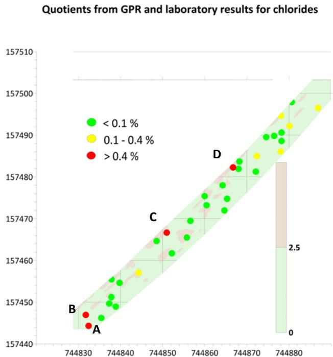
**Figure 7: GPR quotients and laboratory results for chlorides**
