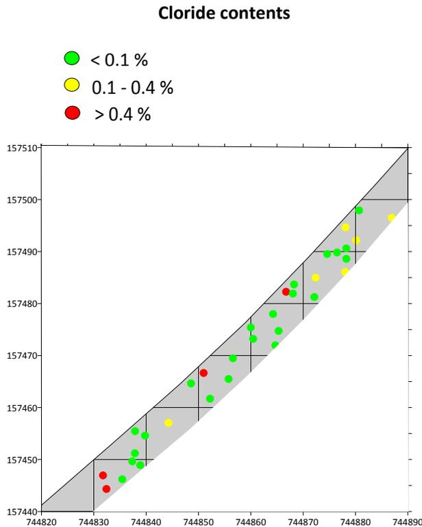
**Figure 6: Chloride contents on bridge deck**
